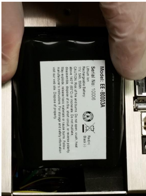
Step 5 – Carefully push battery into the compartment
