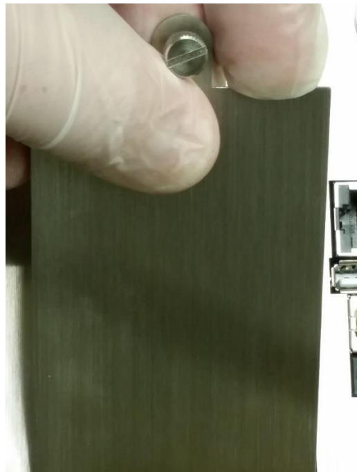
Step 6 – Replace battery compartment door and tighten thumb-turn knurled screw
