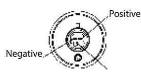
Top View: 3-Pin Packard Connector Type: P2S Series 150
